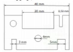
If the hook length fits within the 20 mm horizontal slot, then the maximum body thickness must fit in the 5 mm vertical slot.
